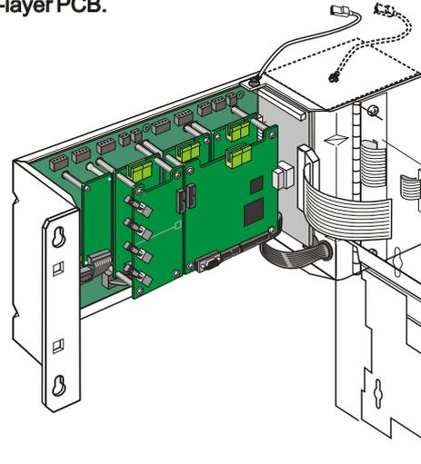
To remove the Fibre-optic PCB, disconnect all fibre-optic cables and ribbon cable (see below) and remove the four retaining screws.
